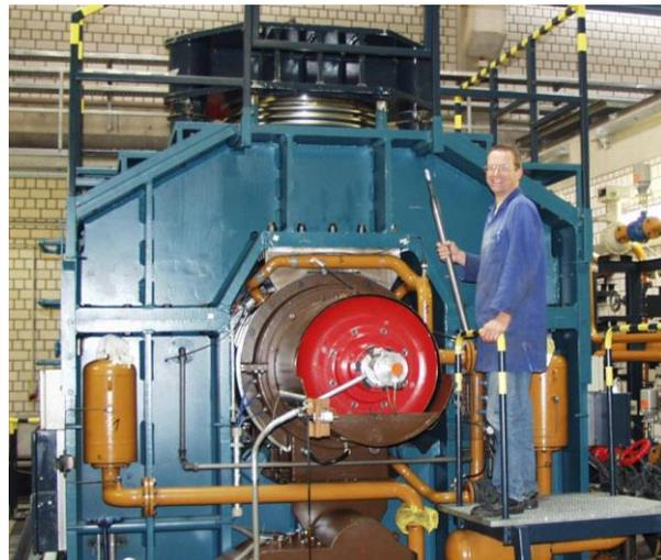
The oil film thickness and pressure sensors are located at the surface of the shaft. Lubrication film thickness and pressure distributions across both circumference and length of the bearing are measured by slowly shifting the rotating shaft in axial direction. The measured data is transferred by a slip ring assembly.
